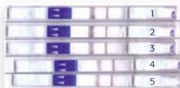
▲ Analysis of rapidPCR amplification products at various dilutions of the starting template using a lateral flow strip (LFS) for detecting influenza A
