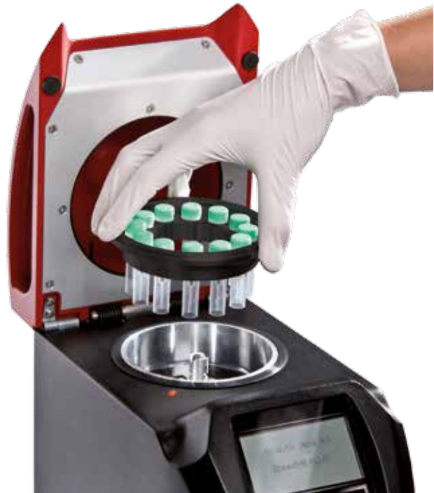
Exchangeable sample adapters enable an easy sample handling
