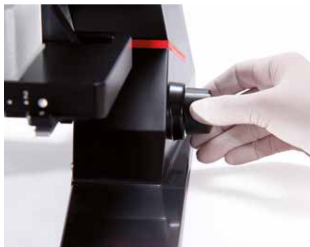
Positioning of the pipetting head and setting the right height – very easy due to the integrated rotary knob.
