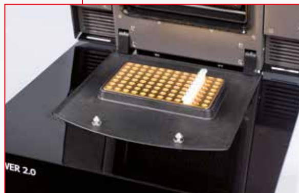
■ qTOWER 2.0 with gold-coated 96 well silver thermal block
