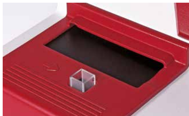
■ Measurement position for 10 mm standard cuvettes
