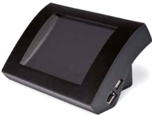
Portable and versatile HID-Pro 320 user-interface with 5.7"color touchscreen
